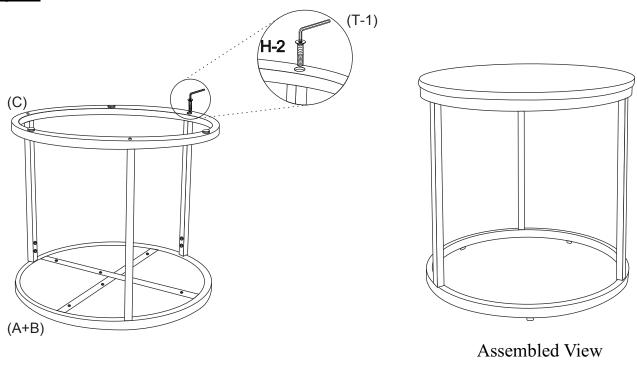
Gently place Bottom Frame (C) onto Legs (B) as shown. Ensure the holes on Bottom Frame (C) are fully aligned and engaged with the pre-threaded holes on Legs (B). Secure Legs (B) using 3 Large Allen Bolts (H-2). Fully tighten all bolts using Allen Key (T-1). Carefully turn the end table upright and product is now ready to use.
