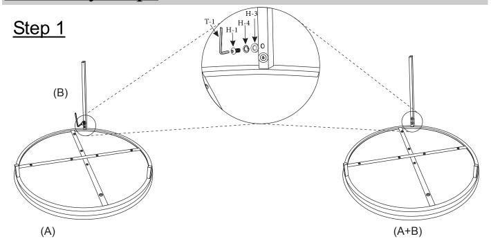
Place Top (A) upside down on a non-marring padded surface. Install leg (B) onto the Top (A) using two Allen bolts (H-1), two washers (H-3) and two spring washers (H-4), stacking hardware in the order shown above. Repeat same steps for the other legs. Make sure all bolts are fully engaged into the pre-threaded holes on the metal blocks. Do not fully tighten all bolts until the entire unit is completely assembled.
